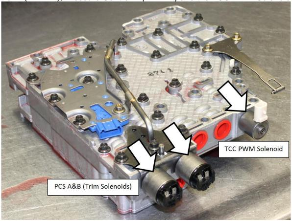
1030471-1030473 – 2004-2010 Allison valve bodies are supplied with four solenoids. Pressure Control A (TRIM A), Pressure Control B (TRIM B), TCC PWM and Main Mod (G Solenoid).
